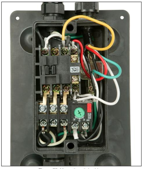
Figure 75. Magnetic switch wiring.
